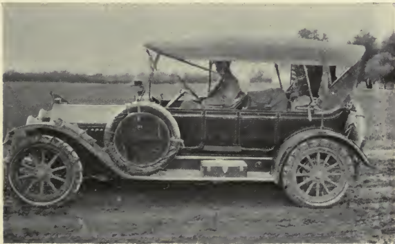
On the dirt roads of the Middle West prairie States it is a wise precaution to use Weed chains on front and rear wheels when the roads are wet
